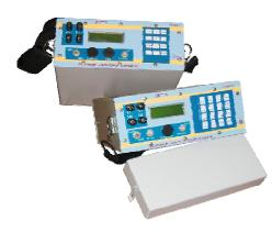
Portable digital electrical exploration system ERP-1 is designed for geophysical survey performed by the following methods
