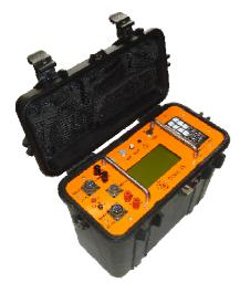
Multinode resistivity meter for 2D and 3D resistivity tomography.
