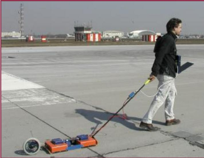
On airport operation and implementation of reconstruction and repairs of runways there appears a number of questions concerning the structure and state of constructional layers of runways, defects and heterogeneity in hard coating and lower coating.
