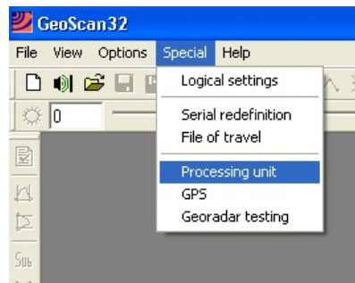
Figure 2.3.31. Activation of file copying window from the CPU
