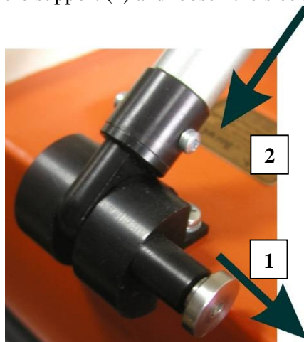
Figure 1.1.6. Fastening of the beam-handle to the AB
