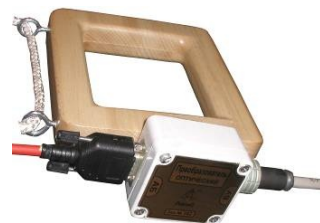
Figure 1.1.13. Optical converter fastening to the transport handle
