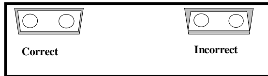
Figure 1.1.10. Optical interface cable connection
