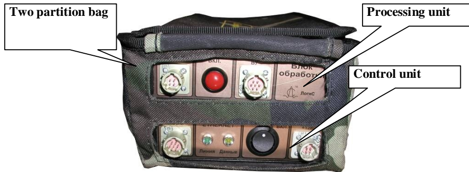
Figure 2.4.2. The control unit and processing unit in the bag
